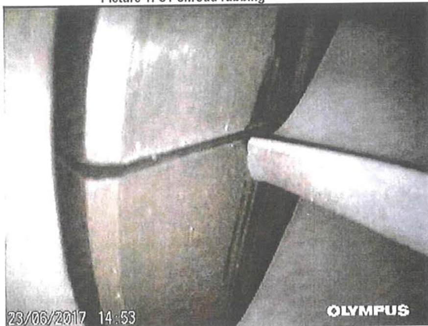
Picture 2: CT shroud rubbing
